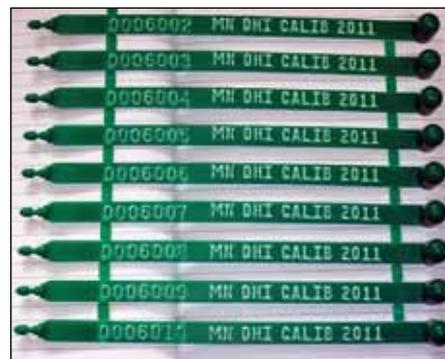
*A calibration tag, such as this one, attached to a milk meter is your assurance that the meter will provide an accurate estimate of milk yield on test day.*
